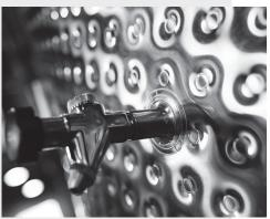
Laser Plate jacketed tank components are a more efficient solution than half-pipe and double wall constructions.
