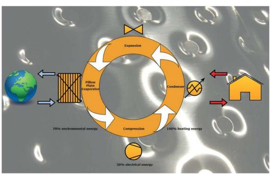
Fig. 1. Refrigeration cycle showing 70% energy savings by using natural heat sinks such as the ocean.
