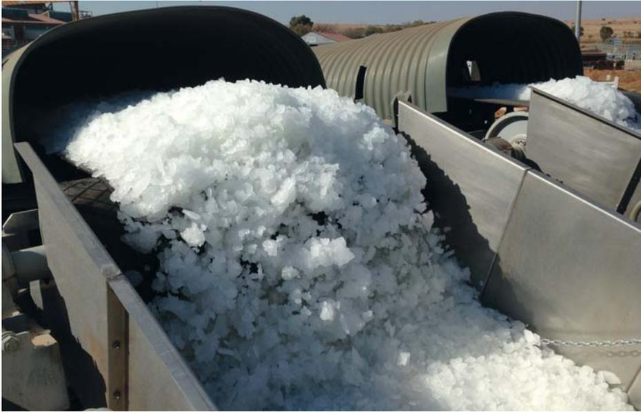
⤴ Fig. 5. Chip ice example from Pillow Plate ice machine.
